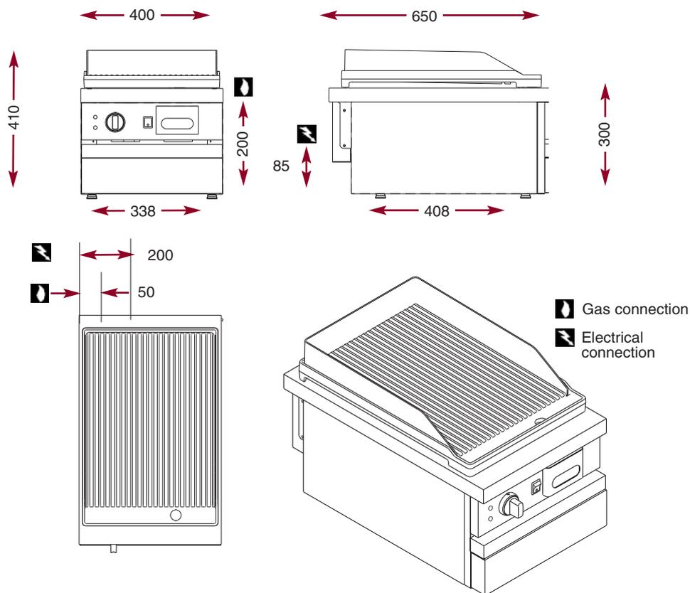
The modules have the same features and performances as the cupboard units. They are designed to be fixed onto tubular steel supports but can also be installed on stainless steel or tiled worktops.
