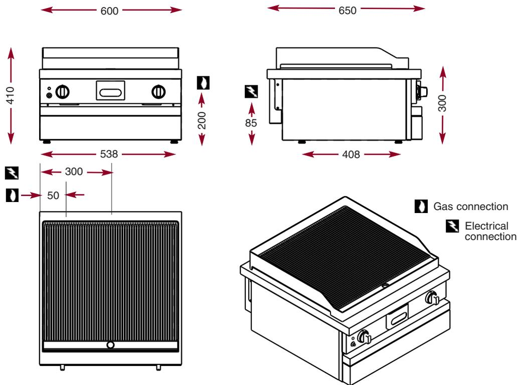
**T**he modules have the same features and performances as the cupboard units. They are designed to be fixed onto tubular steel supports but can also be installed on stainless steel or tiled worktops.
